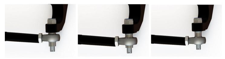
c. Install ARP 12-pt nut beneath the rod end by hand, do not tighten until you've done re-alignment
