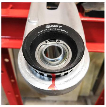
e. Insert and tighten outer joint lock nut using a soft tool and a hammer
