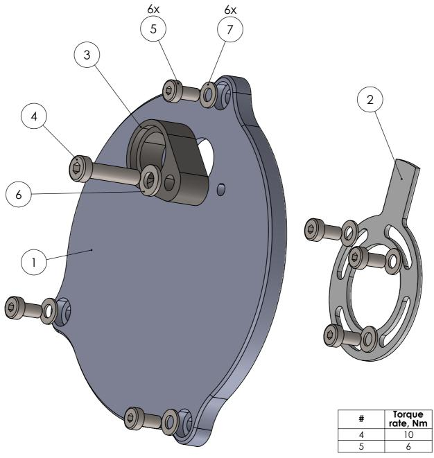
Assemble trigger lever bolts with Loctite
