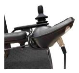
When the indicator light of the charger turns green, unplug the plug of the charger, then pull out the power plug.
