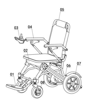
Unpack the wheelchair and locate the charger, tool kit, and spare parts. Install and mount the controller on the right or left armrest.
