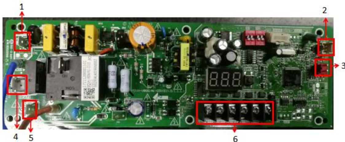
Figure 5-1.1: 28 model outdoor unit main PCB ports
