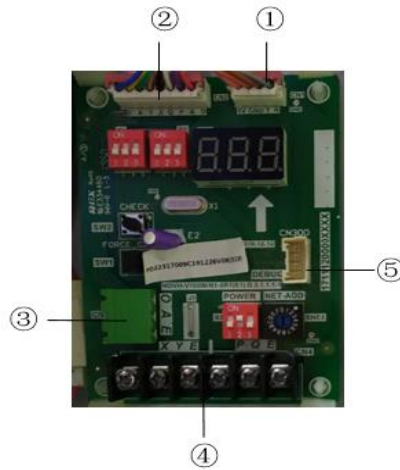
Figure 5-1.3: 36/42 model outdoor unit Communication converter board PCB Ports
