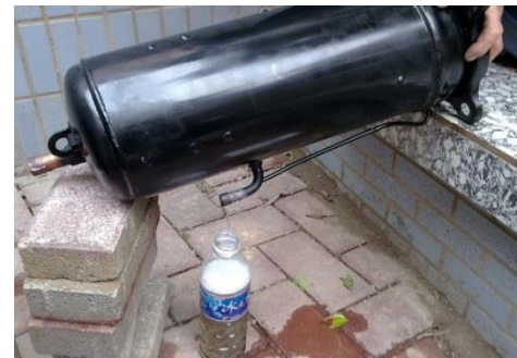
Figure 6-2.5: Draining oil from a compressor
