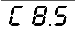
Figure 6. When flashing, the pump is in Time Dispense Setup Mode
