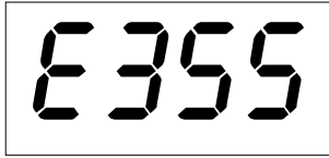
Figure 4. External Control Mode, 355 rpm
