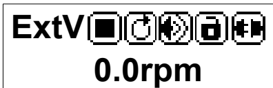
For External Voltage Signal 0-5V/0-10V
