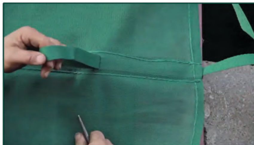
Fig 5 Pulling webbing strap through material
