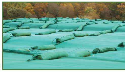
Premium Gravel Bags are **1m long 20cm wide** and made from the unique Secure Cover **250 gsm** knitted HDPE netting. Premium Gravel bags have a side and end handle with overlocked stitching. Each bags is supplied with a cable tie to close the end once filled.
