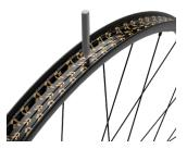
2. Install the valve stem through the rim tape and into the valve stem hole. Thread the nut onto the valve stem from the opposite side of the rim.
