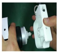
4. Install the left end cap on the plastic part of the spring, rotating it in clockwise direction to add the spring force(rotating 10 laps), rotating it to a jammed point, that is, you feel the spring will not reverse by itself ,then you can release your hand.(when adding the spring force, pay attention to hold the end cap tightly to avoid it turn over and hitting hand)
