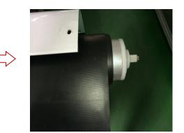
3. Install the left end cap , rotating it in clockwise direction, release the locking, use one hand to hold the axis, remove the end cap to release the spring force. (This step need to be operated twice, to prevent the original spring force didn't remove completely
