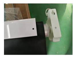
5. Hold the right end cap with hand, pull up the axis with a rope, then at the other end need another person to pull the axis into the housing ,insert the axis into the right end cap inner slot .
