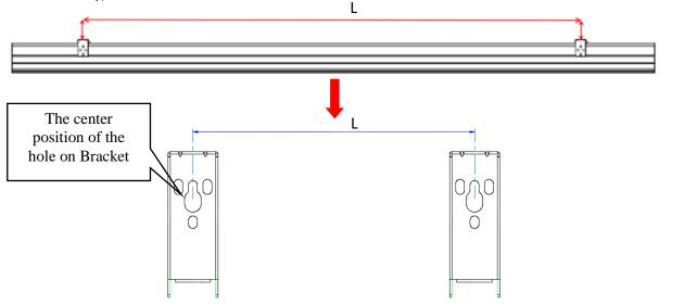
2. Drill the holes and insert the **Anchors** (**E**), and fixed the bracket into the wall with **M5.5** screws(**D**), then loosen the screw under the **Bracket** (**A**) counterclockwise.
