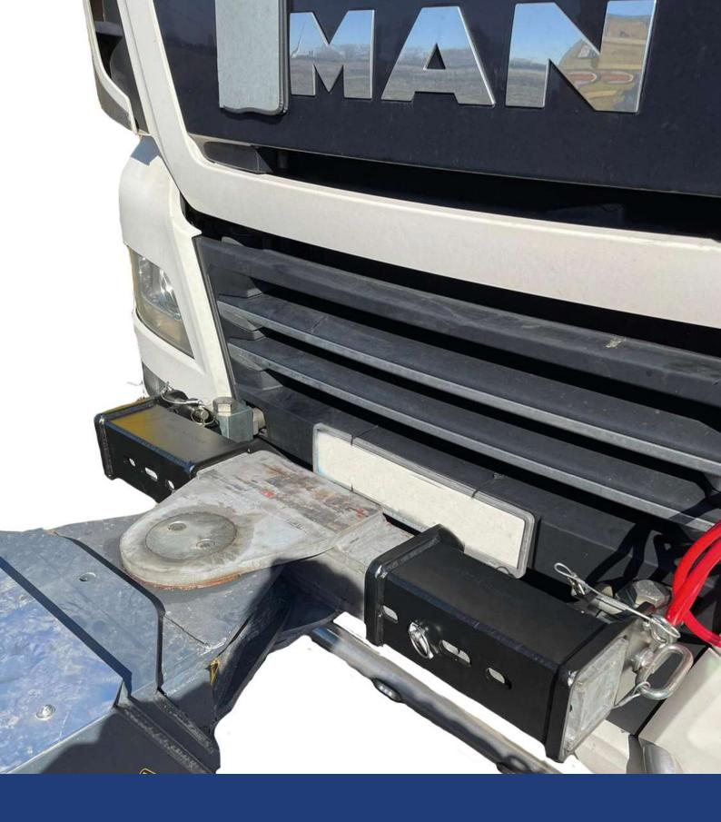
"The Safe-Bar System reduces weight on the recovery vehicle, increases ergonomy, flexibility and provides a better lifting momentum."
