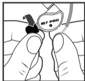
2. ROLL TIP INTO THIN, ROUND CYLINDER
