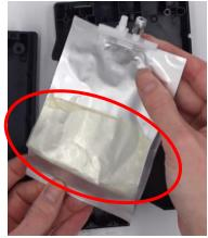
Place the new FIREBIRD ink bag in the chip side of the cartridge with the label facing upright.
