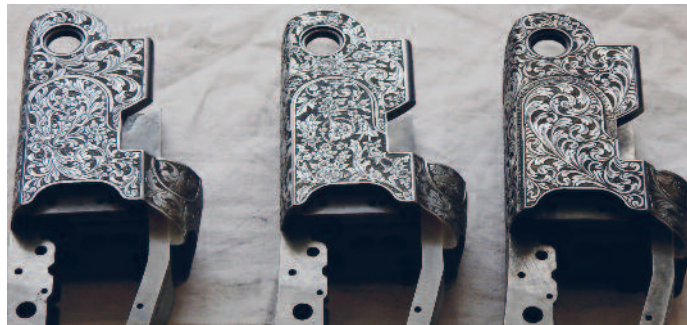
12GA 680 SERIES BERETTA COLE CUSTOM ACTIONS ENGRAVED BY PEDRETTI STUDIO OF ITALY.
