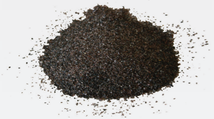
40' brown fused alumina, for sandblasting in stone or for blasting metal structures. Bag: 25 kg.
