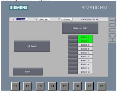
On this screen you can select sandblasting all defined fields or just one field selected from the list. The system will start sandblasting once the choice is made.
