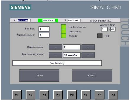
On the screen we can see the currently sandblasted field (in green), sandblasting repetition meter, speed and abrasive level sensor status.
