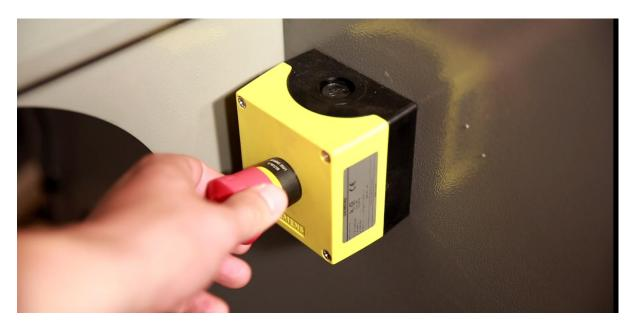
**ATTENTION:** Do not use safety switch in order to stop the sandblasting process without serious reasons. Using safety switch when it is not necessary may result in destruction of sandblasted surface. Safety switch stops the engines and the sandblasting machine, but remains of the abrasive in the cable may still go through the sandblasting nozzle.
