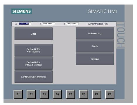
Start sandblasting from defining fields for sandblasting. Start marking fields by pressing Defining fields button. After defining all fields start sandblasting by pressing Job button. All the steps are described in the following sections:
