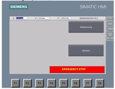
After starting the program, the first thing you need to do is to reset the system position. Information that you need to do it is shown at the bottom of the screen (on the information bar).
