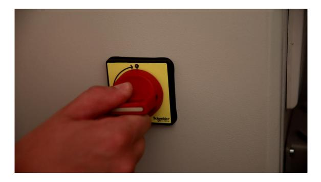
Safety switch is located on the side of the machine.
