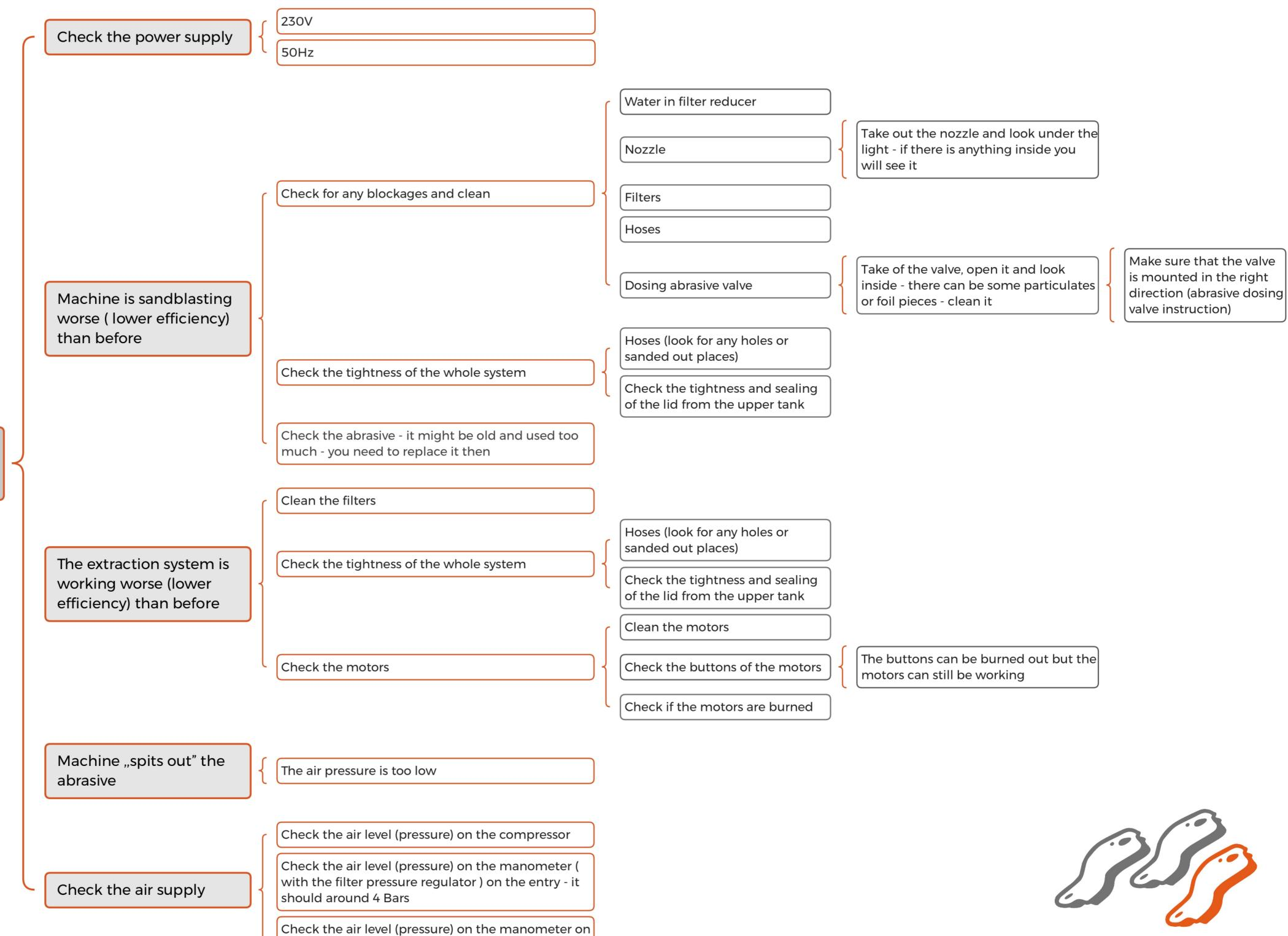
the pressure tank (it works only when
