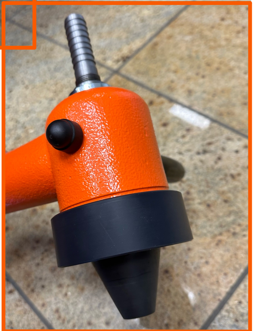
Head with fastening and rubber head cover
