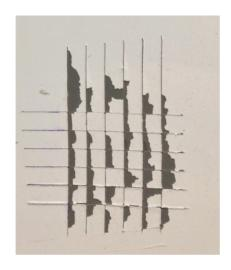
Without the use of software, it would be very difficult to estimate the percentage of coating removed from the image above. However, using a smartphone and a special application, the area removed can be automatically calculated and discovered to be 28%, making the classification rating of this coating a 2B. Also, since the test site has been digitized in order to calculate the amount of coating removed, it is easy to share electronically with interested parties.
