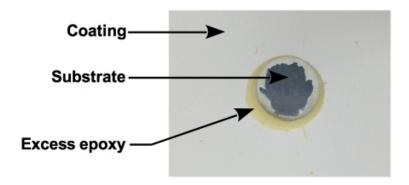
Most technicians performing pull-off adhesion testing would consider the test above a 'good' test. As a matter of fact, in the last round robin session administered by ASTM to develop precision and bias data
