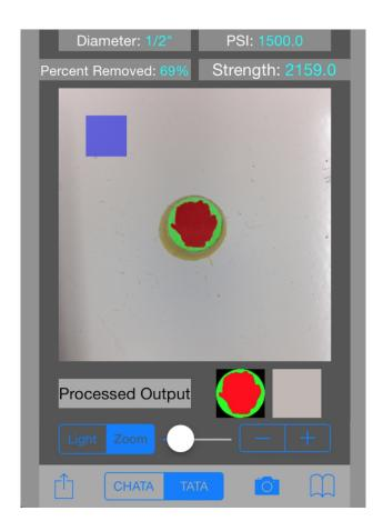
As you can see, using the smartphone's camera and an application the user can properly calculate the tensile strength of their coating using the actual area pulled rather than some ideal, perfect world case. After using the app to obtain an image via the smartphone's camera, the user would then input such parameters such as the diameter of the pull stub and the value returned by the adhesion tester to obtain the true tensile strength of the coating.
