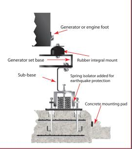
Some state and local codes require vibration isolators that provide protection for seismic or earthquake ground effects. If the generator set is already fitted with integral neoprene mounts, the addition of spring mounts for earthquake conditions should be as detailed. The spring mounts should equal the integral mounts and be located in the skid rails vertically inline with the existing neoprene isolators.
