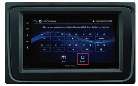
Now, you can begin the learning process for your specific steering wheel buttons. Press each button on SWC settings one by one, making sure to press the corresponding button on your Steering wheel for each one.
