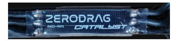
NOTE:- CARBON FIBRE IS CONDUCTIVE PLEASE ENSURE THAT NONE OF THE SOLDER PADS OR EXPOSED WIRES IS TOUCHING THE CARBON FIBRE FRAME PLEASE USE INCLUDED HEATSINK TO INSULATE ALL CONNECTIONS FROM THE FRAME.
