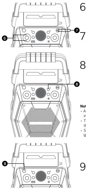
Press the MIC VOLUME + or button as desired, which will affect both microphones.
