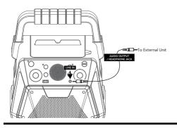
Connect an external device by using an appropriate cable (3.5mm audio cable not included) as shown.
