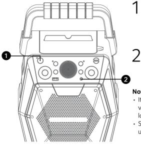
Connect the unit as described previously. Press the **ON/ STANDBY** button to turn the unit on.
