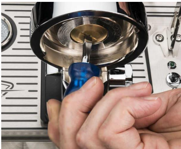
Figure U 8. Remove dispersion plate from group head.
