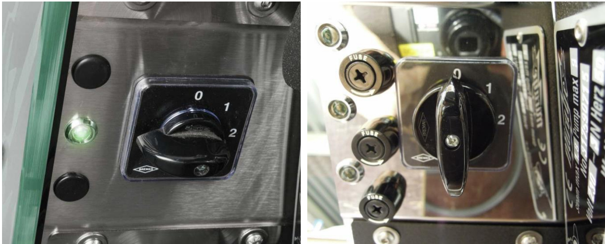
Figure U 1 (left). Showing the mains switch of a Duette with its 3 positions: “0”, “1” and “2”. Indicator light is lit meaning that heating element is “on”.
