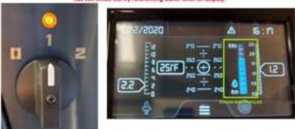
If reachine has timed sur, cycle machine aff/on (position "1") again and allow to auto fill. If machine is still timing out, shut machine down and to check the inlet water line / filtration system and confirm water flow to machine.
