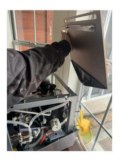
Watch for the electrical connection! Make sure to detach the connector.
