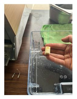
Remove the metal clip and the magnetic float.
