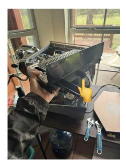
You may remove this cap from the drain bin to add a hose for an external drain.
