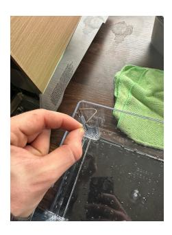
Press the metal clip most of the way into the corner.
