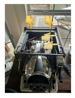
Next, remove the 4 Phillips screws holding on the side and rear panel.
