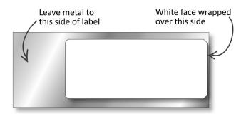
Smallest recommended bending diameter of the Confidex Silverline Blade  $\Pi^{\text{TM}}$  is 100mm. For optimal performance please bend the label in the orientation shown below.
