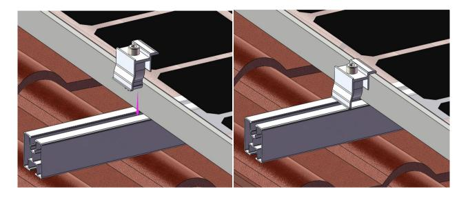
Midd clamp installation: as shown in the picture, press the Midd clamp into the card slot, lock the bolt, and press the panel
