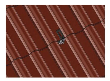
Repeat the preceding steps to install all hooks. Ensure that the top surfaces of hooks in the same row are at the same height to ensure the normal installation of guide rails
