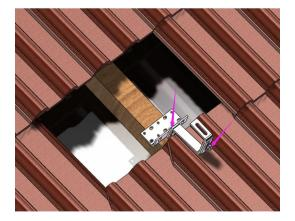
Locked to wooden beams with wood screw hooks. Generally, one hook locks three wood screws
