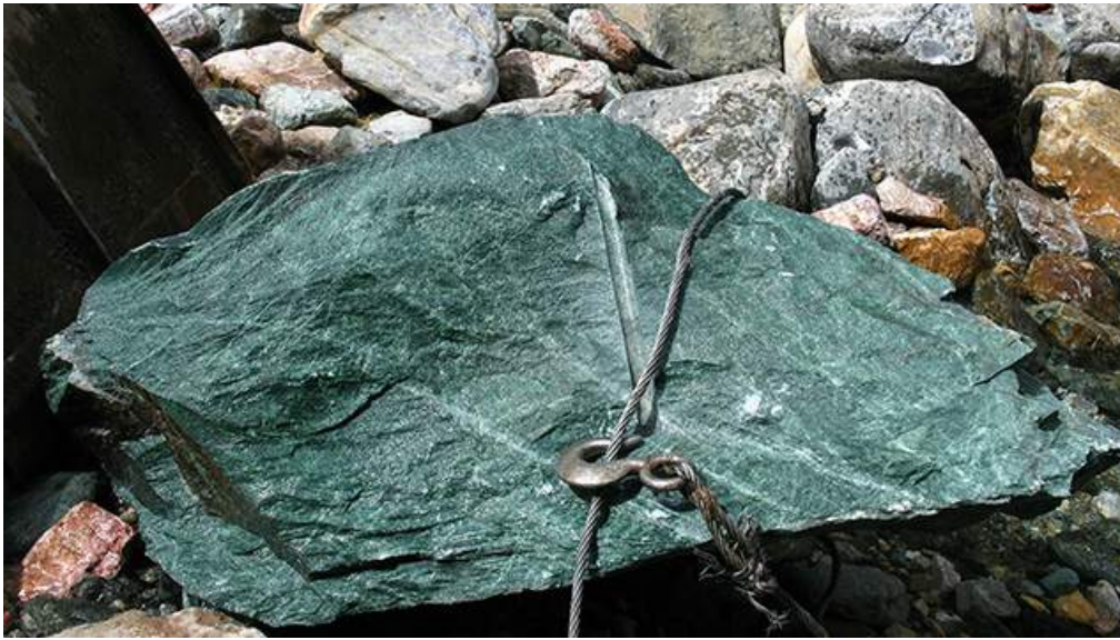
In 2009, miners found a nearly five-ton green nephrite boulder along the Arahushun River in Siberia. Expansion agent was placed in the boulder, and after a year, miners split the cracked boulder into smaller pieces and transported them to the town. Photo courtesy of Jade Factory and Jade Mountain.
