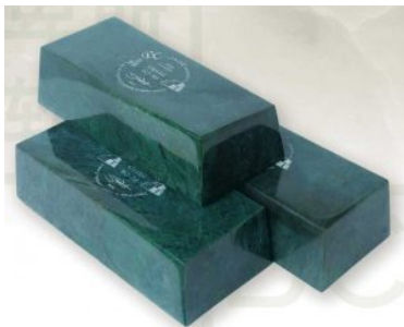
The B.C. Jade Standard is a 10-kg rhombohedron calculated using the known geological density range for nephrite. Its proprietary dimensions meet the requirements of the world's jade jewellery manufacturers.
