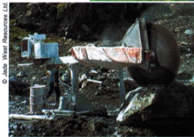
Diamond-tipped saw, cutting jade boulder
