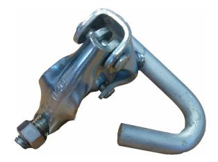
The Internal Scaffold Hook Tie Coupler is suitable for both the 3.5kN & 6.1kN load classes as described in the TG4:11 Standard.
