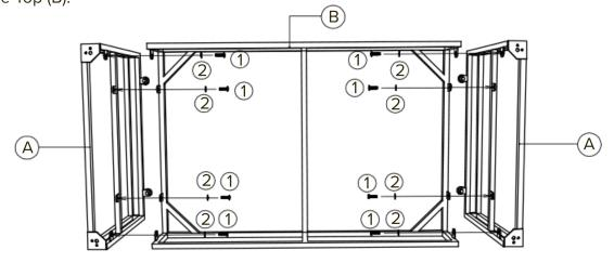
Secure a spring washer (2) and a bolt (1) with supplied Allen key (5).
