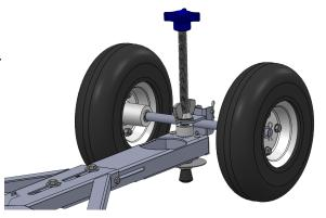
6. Next, attach the Tow Handle (Q) to the Steering Axle (O). Start by taking the handle and align the bottom holes with the side holes in the steering axle. Use the Clevis Pin (M) to keep in place. Put a Cotter Pin (L) through the clevis pin to keep it secure.
