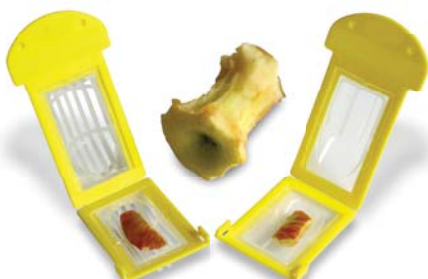
Open and Closed Cage Frame devices with apple samples for testing (not included)
