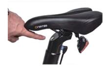
**Activate / Desactivate the battery :** To use **NOMAD**, the battery must be switched On. **When NOMAD is parked, the battery must be switched off.** Press the button on the top of the battery to alternatively turn the battery on or off.
