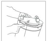
**Step 8**Place lid back to its proper position by aligning the arrow with the rear seam.
