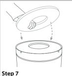
Put back the felt pad removed in Step 4.
