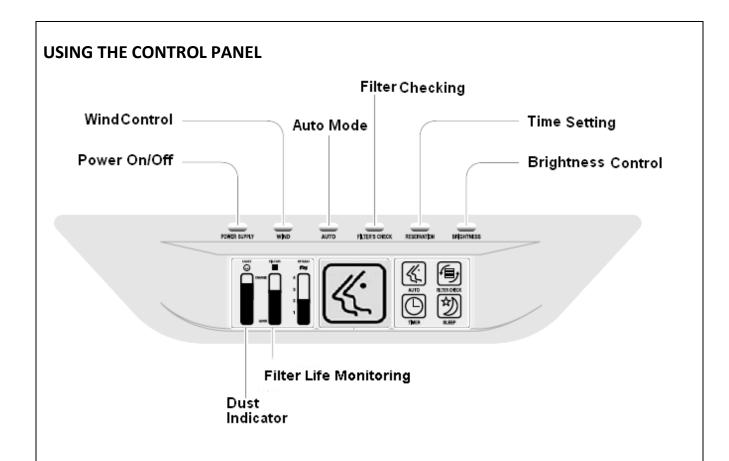
The Airgle 750 Air Purifier is equipped with a state-of-the-art control panel. All controls for the unit are located on the top of the unit. This advanced control panel allows the operator complete control over the unit and provides simple system checks to ensure the performance of your air purifier.
