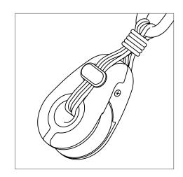
**dynablock** is also suitable for a standing lashing with a thin dyneema line
