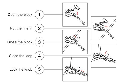
Dynablock is a snatch block with a snap loop for a fast, easy and safe linkage.
