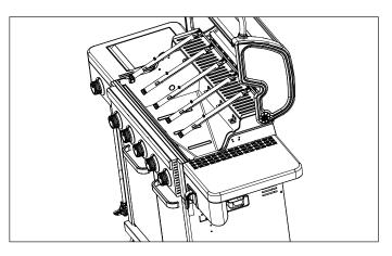
Lift burner up and carefully pull away from front of BBQ. Note Piezo ignition and lead will still be connected. (Fig. 17)
