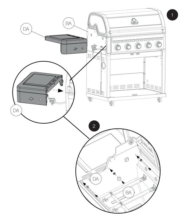
Secure Side Shelf Brace - Left (DC) into Cooking Frame using 1 x Bolt (1), 1 x Washer (6) and 1 x Nut (7).
