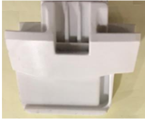
Slider bar end cap does not have a rubber bumper
