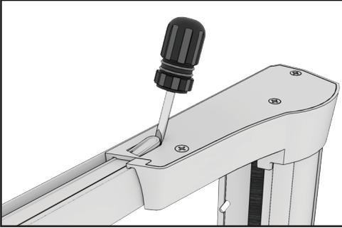
**a.** Disconnect top and/or bottom tracks from screen housing end caps by inserting a flat screw driver under U-shaped tab then pull track out.
