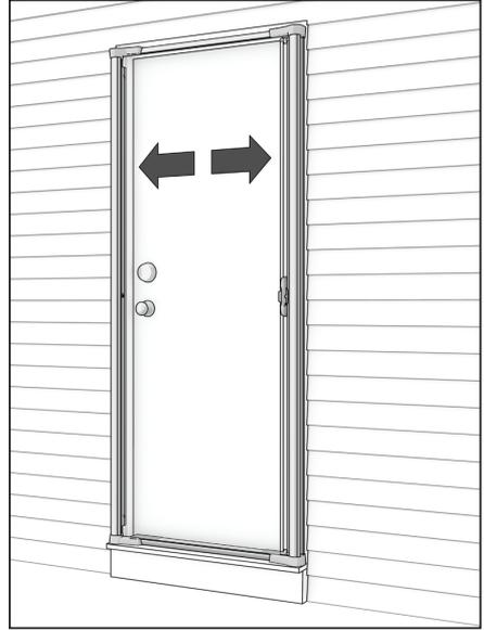
**c.** Secure screen to the opening by inserting a housing screw into the predrilled screw hole at the top of screen housing flange to hold frame in place. Do not tighten completely.
