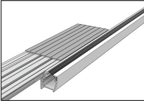
**b.** Remove sill plate from bottom track (if needed)
