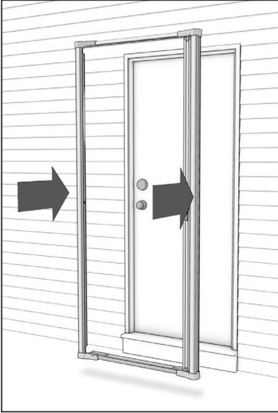
**b.** Extend housing to left and right evenly until both flanges are snug to the edges of the door jamb.
