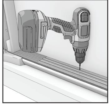
f. Insert housing screws into all remaining pre-drilled holes on each vertical housing flange (2 total per side). Tighten all screws.
