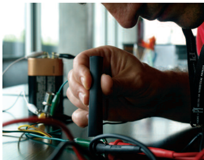
Figure 8: Looking at an LED through a viewing tube.
