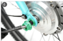
6. Place two gaskets and front fork as shown. Put front fork between two gaskets.
