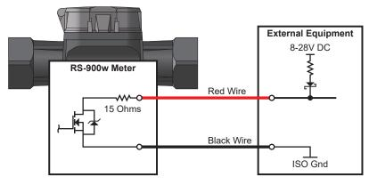
The output of the flow sensor is essentially a 15 Ohm switch with a 600  $\mu$ A current. With no flow running, the flow sensor will appear to the controller input as a small current load. When the flow rate is above the minimum threshold, it appears as a quick series of 5 millisecond connections to ground.
