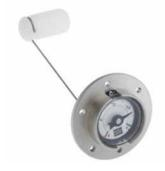
The **G/LL28 Series** is a simple, robust, mechanical liquid level contents gauge using a float to move the dial pointer via a magnetic coupling. This prevents ingress of the tank contents into the indicator capsule.
