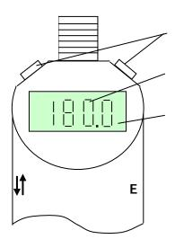
2 keys (↓↑ and E) for adjusting the switch points, switch-back points and additional functions
