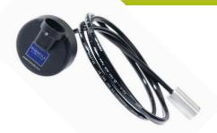
The **T/LL200** series is designed for use in vented tanks requiring continuous level measurement of their contents and provides a factory set linear\* voltage or 4-20 mA output suitable for connecting into a PLC or process related applications. (The **T/LL200** is not a loop powered sensor).
